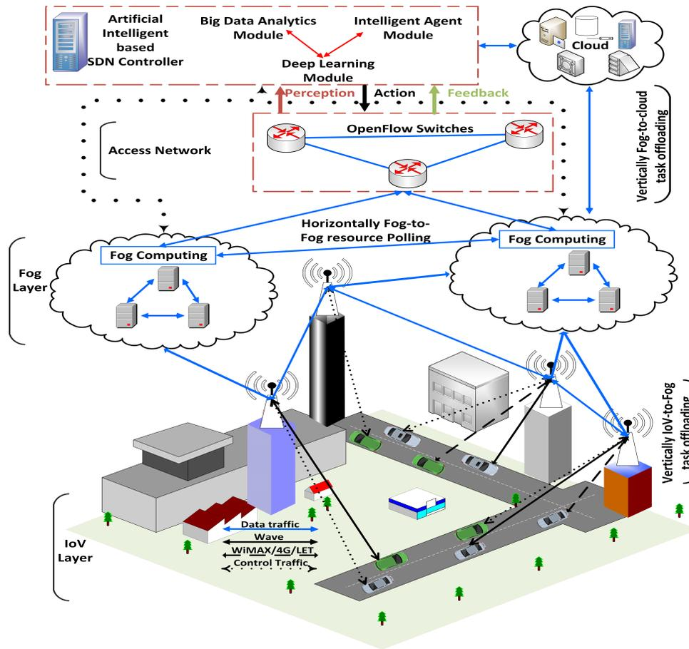
Fig. 1: System Architecture based on ARTNet Model
