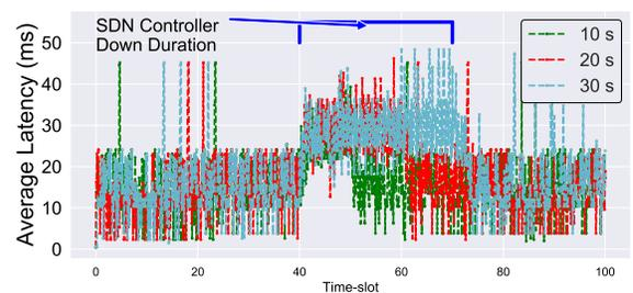
(b) SDN controller failure with Secondary Agents
