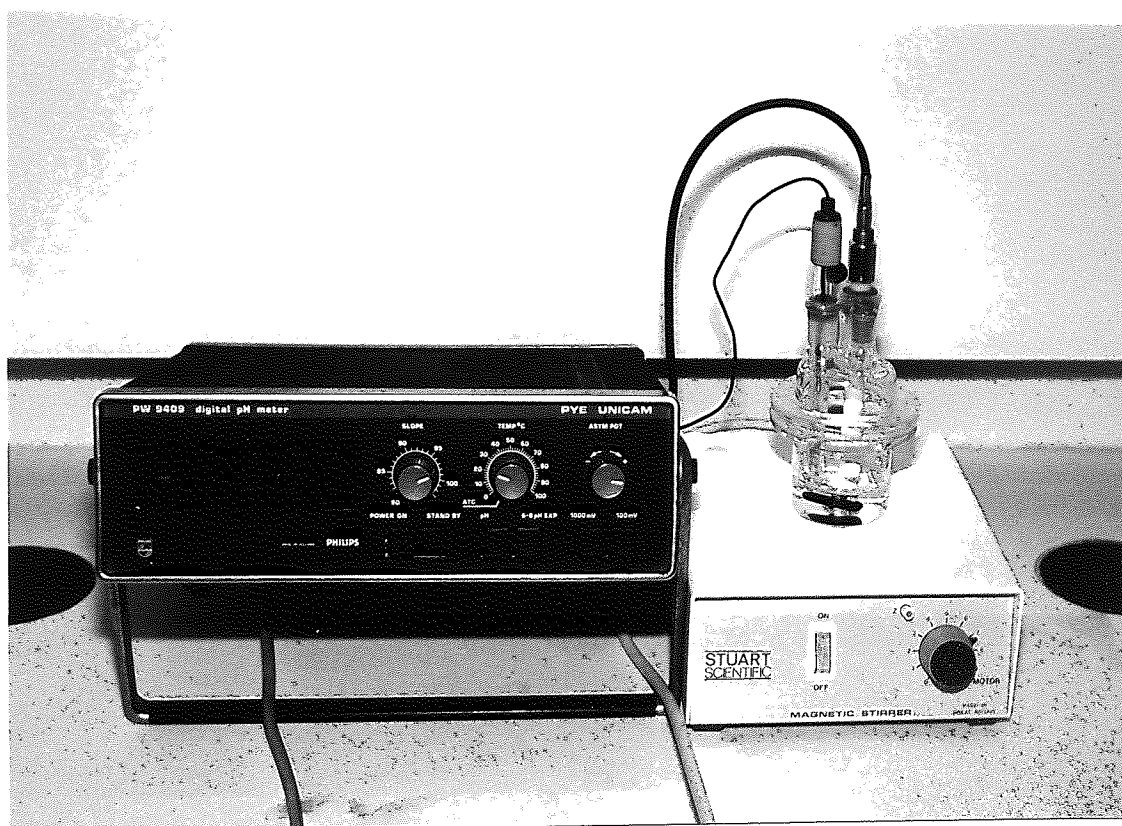
Figure 38 Sulphide ion selective electrode in cell with reference electrode. The cell is shown on a magnetic stirrer to the right of the high impedance voltmeter
