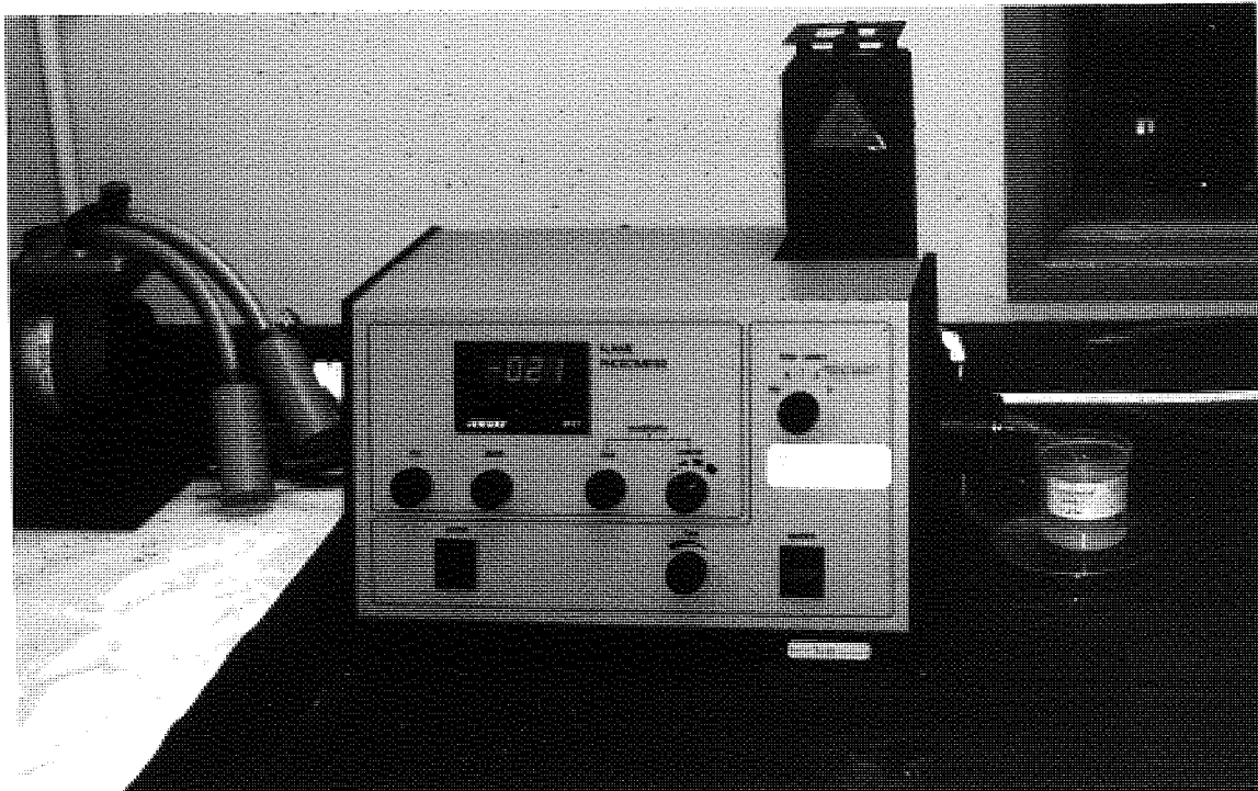
Figure 42 Flame photometer used for metals analysis
