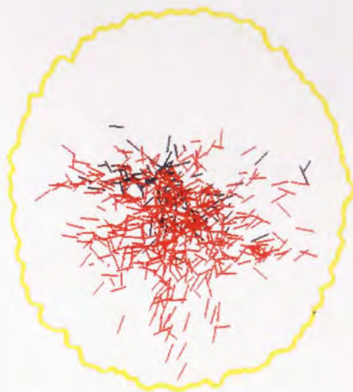
(b) double impact test, 0.2 m/s impact velocity, M_p=M_a : the first 417 bonds broken in the top half and 106 in the bottom half of the agglomerate.
