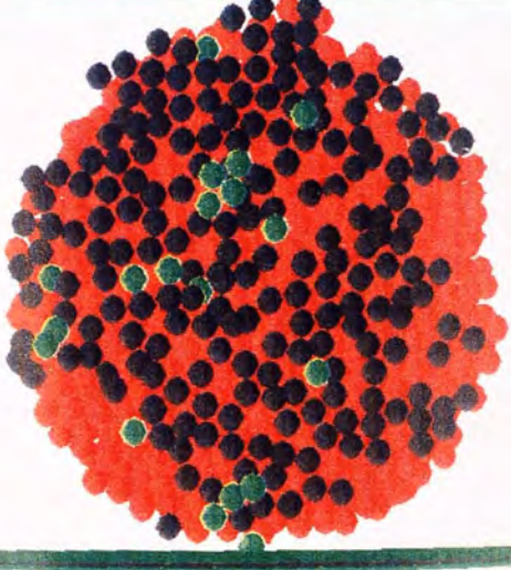
State {6}: t = 8.07 ms (just after secondary fracture). Number of particles that have lost contacts with the largest fragment: 202 (91.4%).
