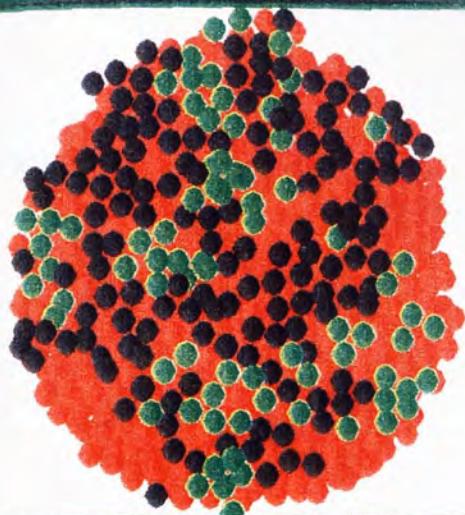
State {4}: t = 8.048 ms. Number of particles that have lost contacts with the largest fragment: 144 (65.2%).
