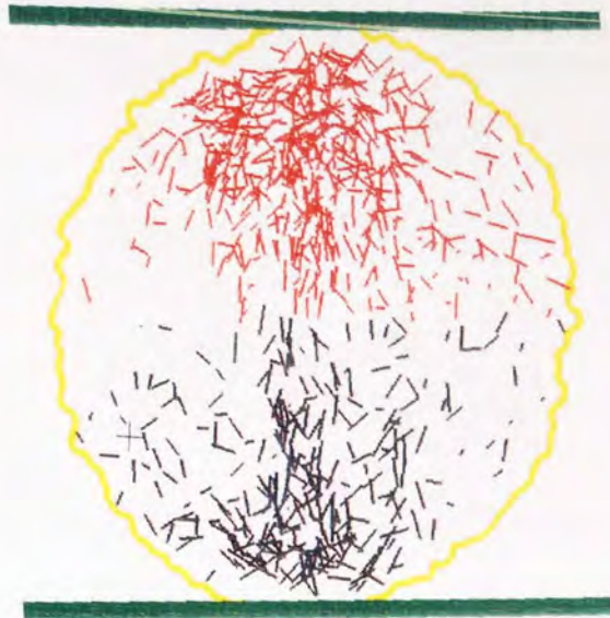
State {3}: t = 0.111 ms - maximum platen force (strain = 0.169%, broken bonds: 2.89% in bottom half + 4.75% in top half of the the agglomerate)
