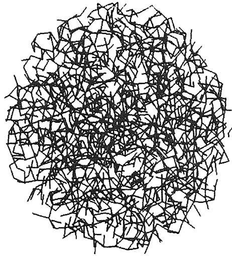
(b) The 1960 tensile bonds in the bottom hemisphere, dense[1] agglomerate.
