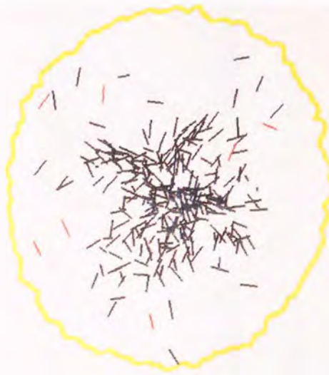
(d) free-fall impact test, 0.3 m/s impact velocity: the first 282 bonds broken in the bottom half of the agglomerate.
