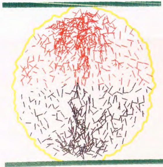
State {5}: t = 0.115 ms - immediately after primary fracture (strain = 0.174%, broken bonds: 3.68% in bottom half + 5.05% in top half of the agglomerate)
