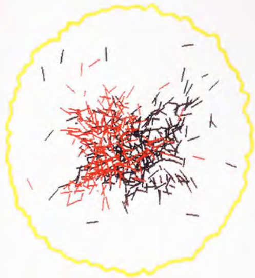
(a) double impact test, 0.02 m/s impact velocity, M_p=100 M_a : the first 197 bonds broken in the top half and 299 in the bottom half of the agglomerate.
