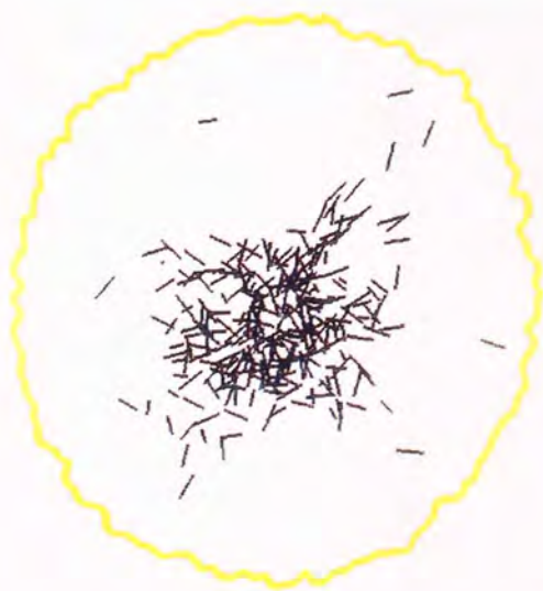
(c) free-fall impact test, 0.12 m/s impact velocity: the first 263 bonds broken in the bottom half of the agglomerate.
