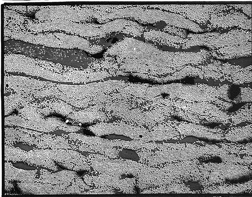
Fig 113. SPECIMENS PRECURED AND MOULDED IN A VACUUM FOR VARYING LENGTHS OF PRECURE
