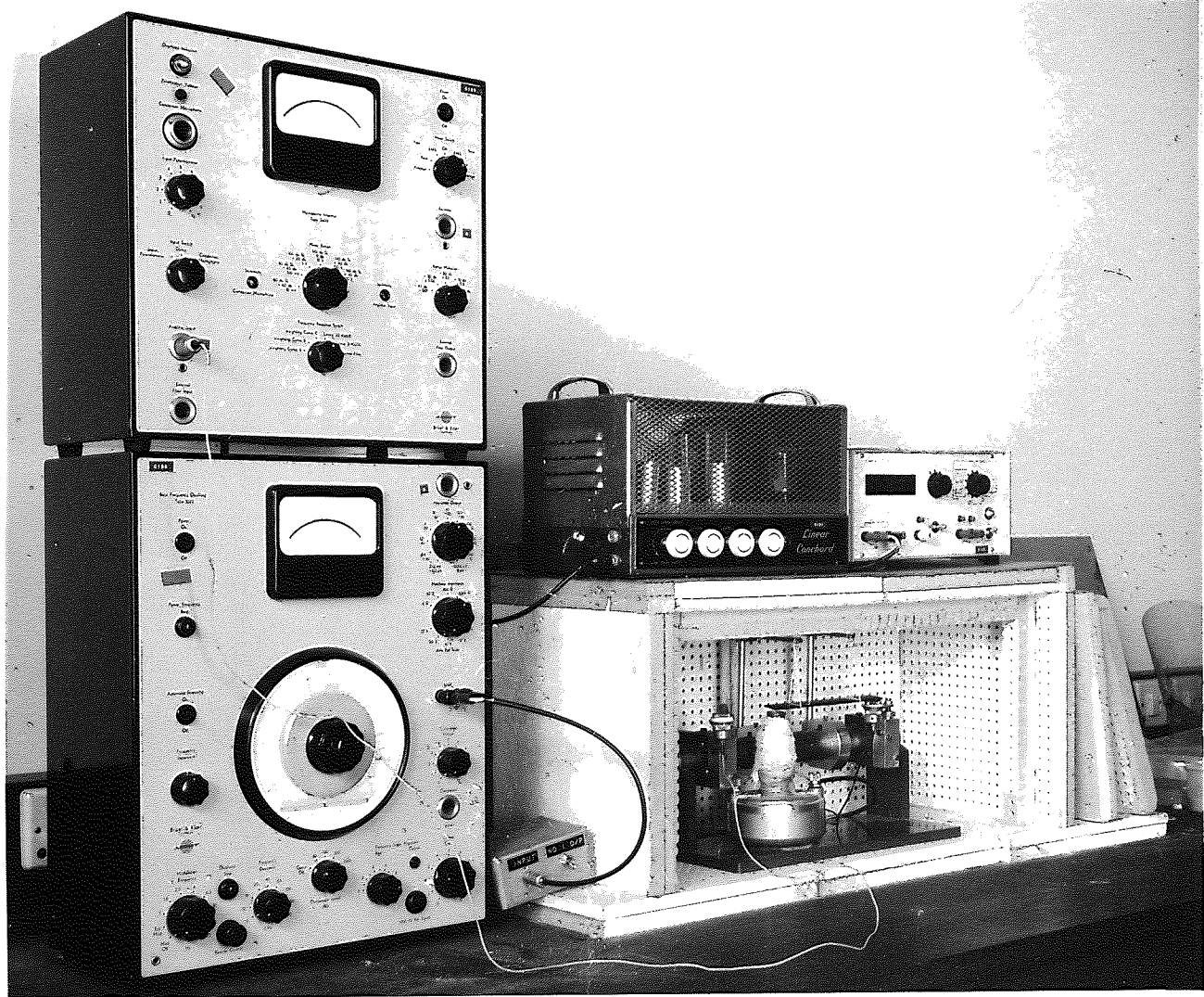
Fig.105. Bruel and Kjaer complex modulus apparatus .
