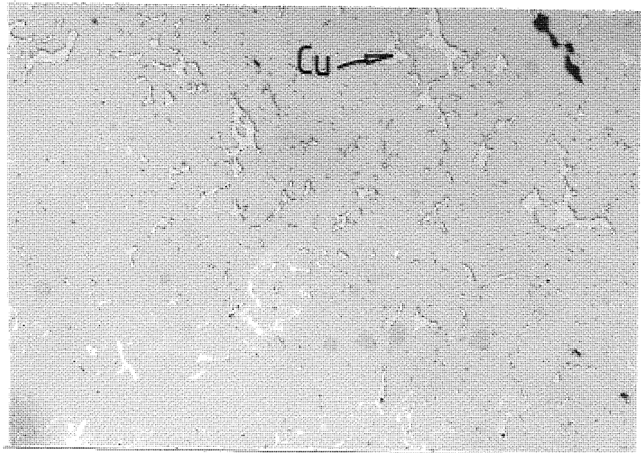
a) Two step infiltration x196
