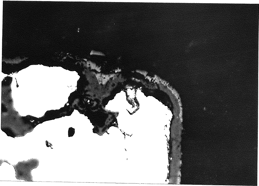
a) Edge and top surface, showing the duplex layer x 980
