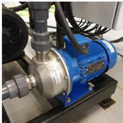
**Fig. 3.7.** Low-pressure pump.
