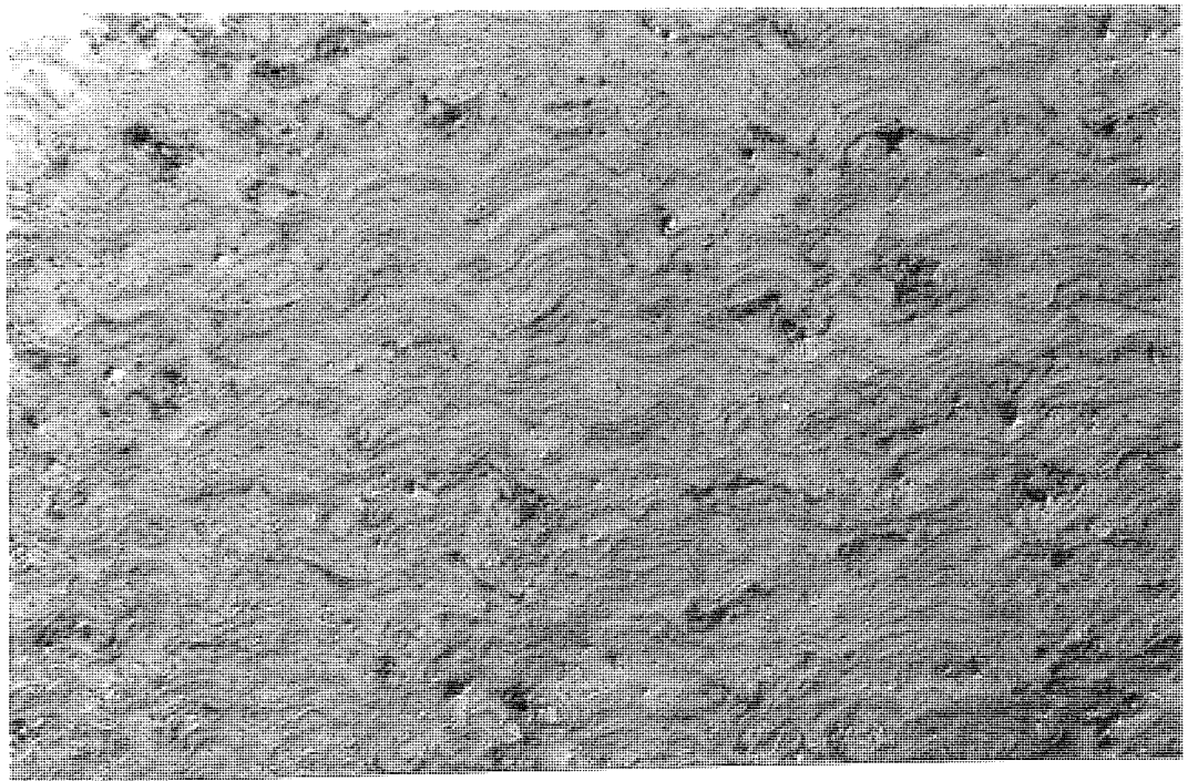
Figure 56. H.S.G. Sample 06A Polarized to show harder oxide bands in relief X 180.
