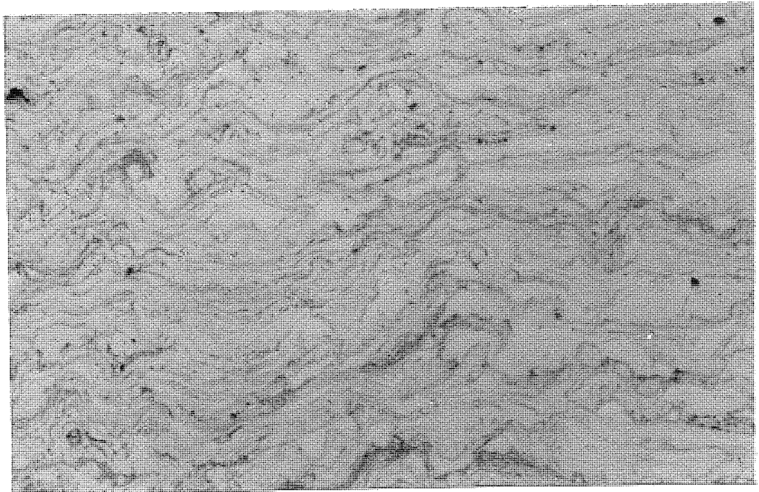
Figure 54. H.S.G. Sample 04 Showing good dense area X 180
