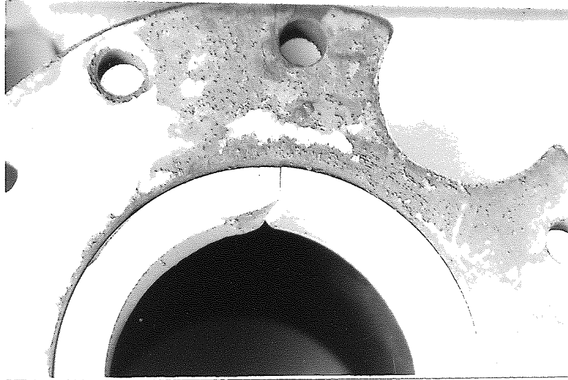
Figure 23. Cracked ceramic liner trapped in outer shell.
