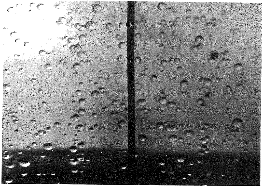
Figure 9.6.7 Exit drops Octan-1-01/Water 0.2% phase ratio
