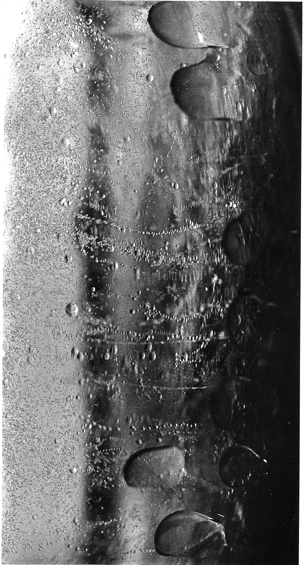
Figure 10.2.2. Mechanisms of release "DRIP-POINT" + "JETTING" + "POINTING"
