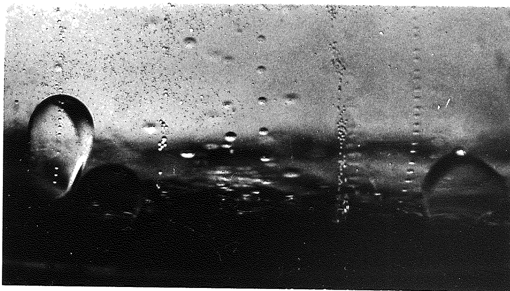
Figure 10.2.6 Mechanisms of release "JETTING" + "POINTING" + "DRIP POINT"
