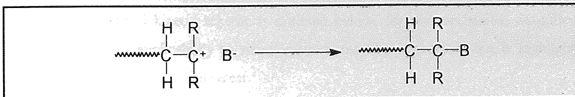
Figure 1.10. Termination by combination of cation and counter-ion.
