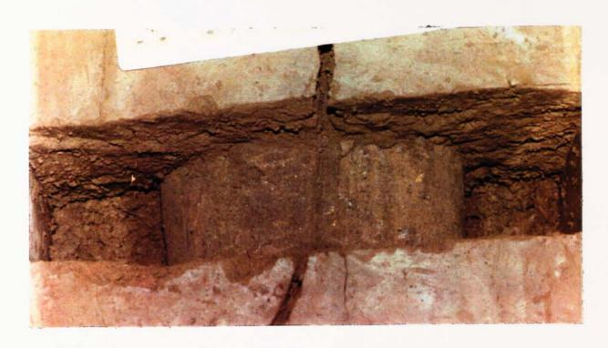
PLATE 8.2 Photograph Showing the Shape Frozen Annulus above the Pipe and the Ground Crack Above the Annulus at the end of the Final Validation Test.
