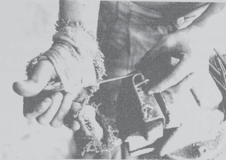
Figure 60. 'Safety glove'. Existing mass produced safety gloves do not allow such delicate movements.
