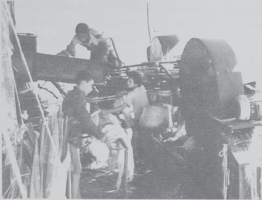
Figure 72. Processed sisal is picked from conveyor belt and then separated to be weighted.
