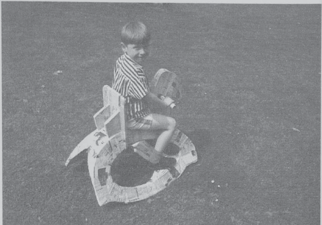
Figure 109. Prototype was then covered with newspaper or cloth to improve finish.
