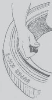
Figure 26. The interior steel ring of the tyre is cut out using a knife to cut it.
