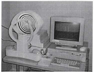
Figure 4.4 Eyesys 2000 Corneal Topography System.
