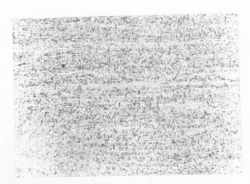
(b) Light etching 'veins'; aged 550°C. Etch; Acidified ferric chloride, X 200
