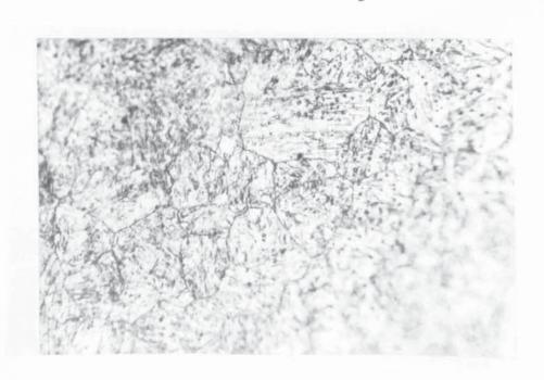
(b) Welded. Electrolytic polish/etch. X 1400
