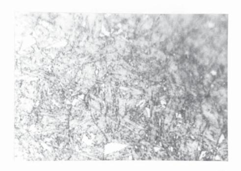
(a) Showing dispersed delta-ferrite; also pinning of grain boundaries by small precipitates. Aged 450°C. X 2,000
