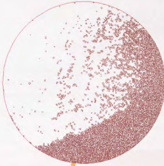
Figure 3.13: 'cir' image of the bed cataracting, \omega = 12\text{rad/s}
