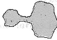
Figure 5.2: Illustration of solid bridges between two particles in a granule
