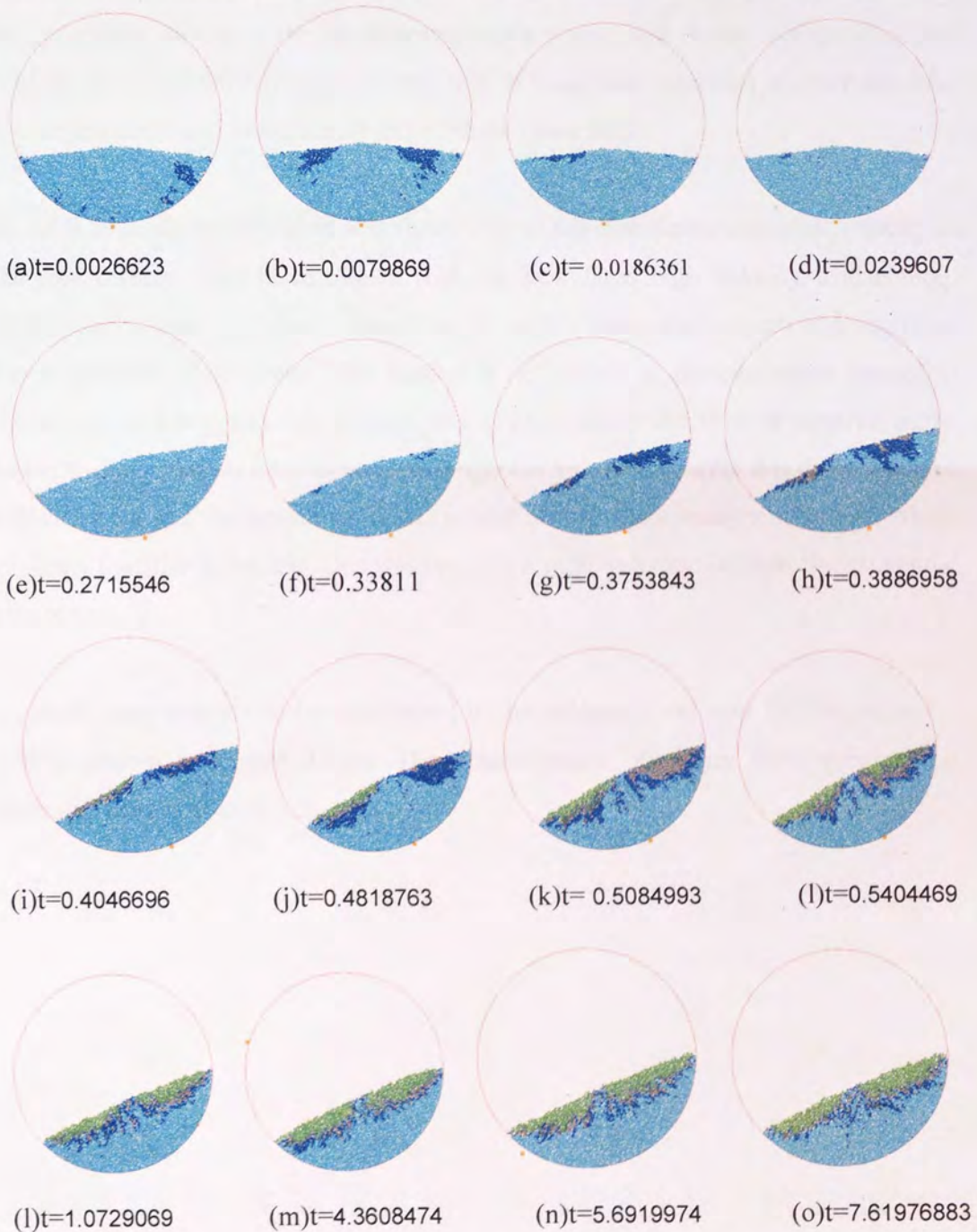
Figure 4.3: Snapshots taken from the radial speed/velocity animations for the drum
