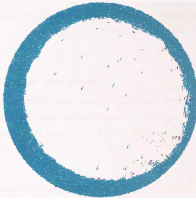
Figure 3.17: Velocity field of the centrifuging particulate system, \omega = 20 rad/s [Maximum velocity = 1.51m/s, Average velocity = 1.36m/s]
