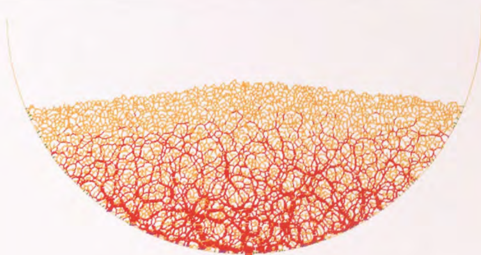
Figure 3.7: Connection diagram of the settled bed. [Maximum force = 3.93mN, Average force = 0.388mN]
