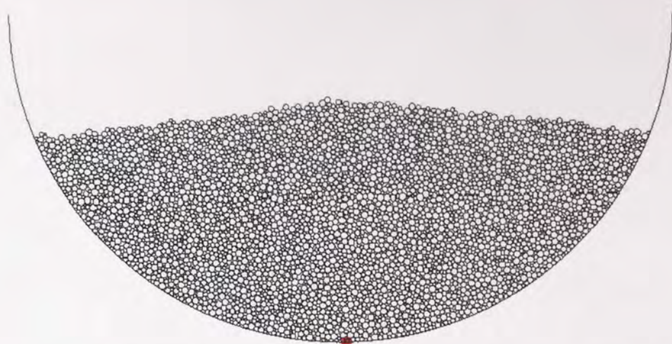
Figure 3.6: Settled bed at time, t=0.8s , when equilibrium is established
