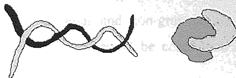
Figure 5.4: Interlocking of two strands of fibres and of two particles.
