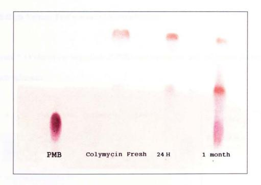
Figure 5.12 TLC separation on silica gel G plates developed with acetone: water: acetic acid: 2 N ammonia (15:5:1:2). Samples: 1, PMB; 2, colomycin freshly prepared; 3, colomycin after 24 hours at 4 °C; 4, colomycin after 1 month at 4 °C. 2 µl of 5 mg/ml solutions of each sample were applied to the plate. The plate was visualised by spraying with ninhydrin and heating at 100 °C for 5 min
