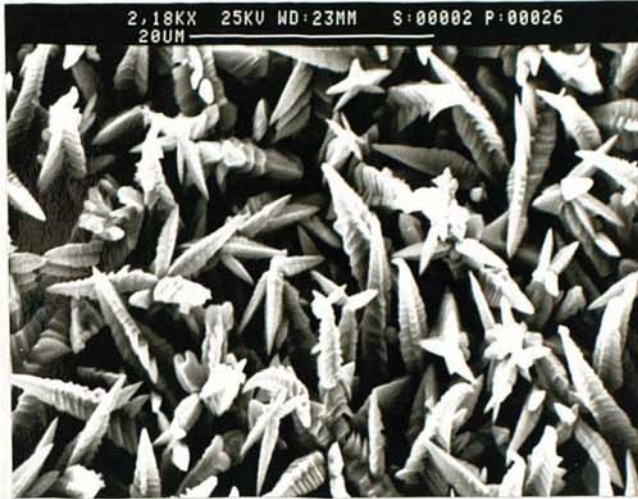
Figure 62. Surface Topography of Deposit Produced Using Cathodic Pulse Time 10 ms, Anodic Pulse Time 2 ms
