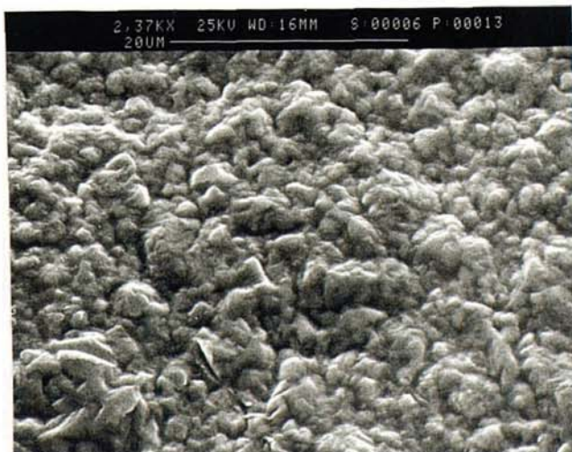
59b) Electrolyte + 75 ppm Oxilube 50,000.
