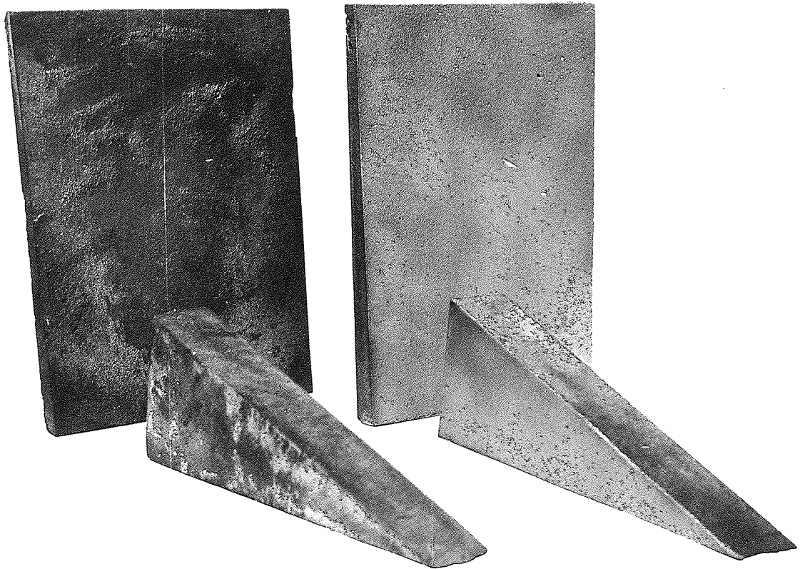
Figure 16.— Showing chill techniques investigated in Series II. These are Cast Iron tapered plate and double thickness single taper chill; similarly in Aluminium.
