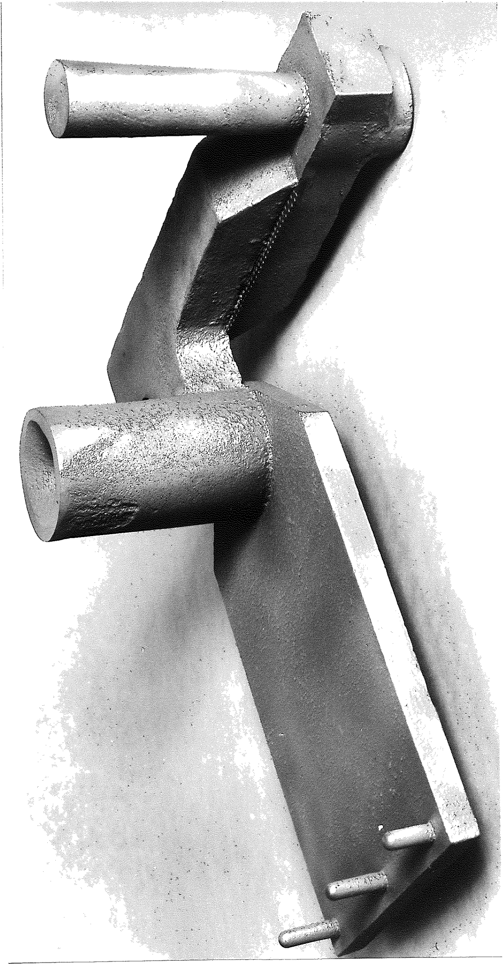
Figure 19.—Showing the final experimental casting shape developed from the work of Latimer 41 and Flemings 43,49 .
