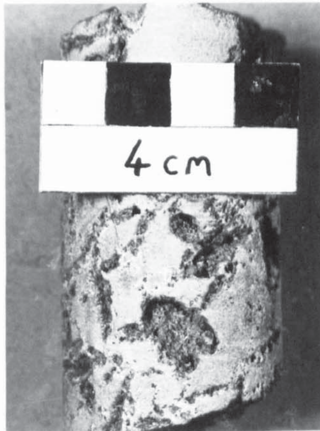
Plate 3.2b Moulds after gypsum seen in unit B of the Ore-Shale. A mould after a swallowtail twin can be seen towards the base of the core.
