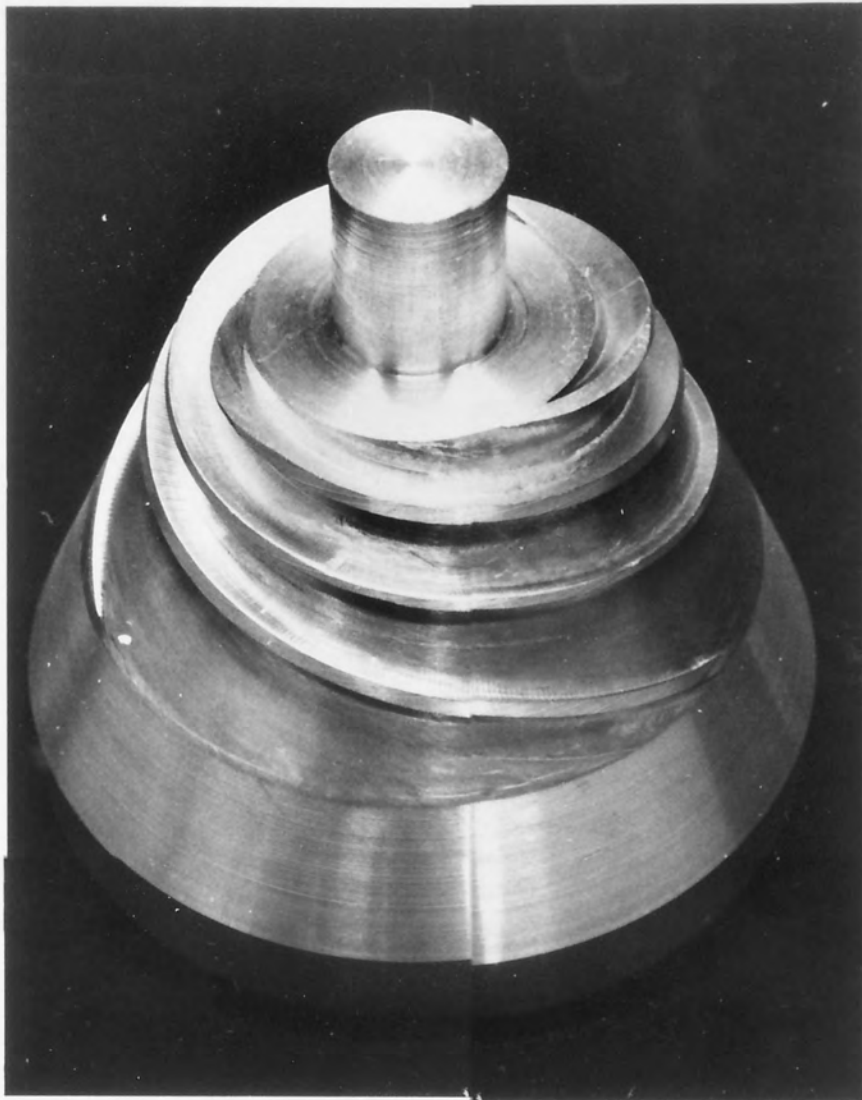
Fig. (6.13) Impellor Cut Using the Fourth Axis
