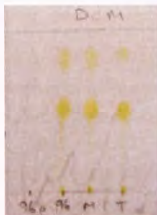
Picture 6: TLC analysis of 96 after attempted tritylation. Left to right; precipitate; filtrate; mixed lane; trityl chloride. Mobile phase: 100 % DCM; visualisation 100 % TFA.
