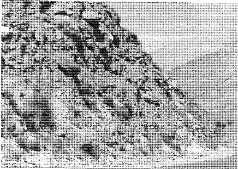
Plate 4.5 Rock fragment flow (km 63). The flow measures approximately 300 m across and 300 m downslope with rapid angle (45 degree) in the toe.
