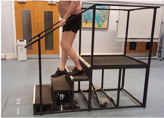
Fig. 1. Staircase with a step height and length of 185 mm and 280 mm, respectively.
