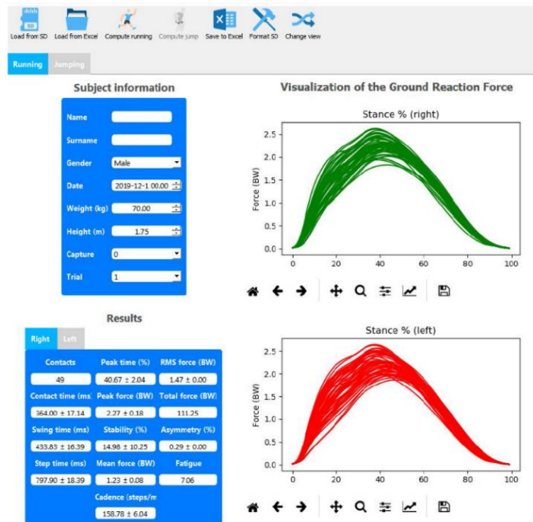
Figure 12. View of a processed running trial showing GRF curves for each stride and running metrics for both legs.
