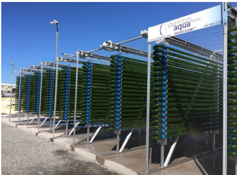
Figure 2.2. Medium scale tubular photobioreactor at Varicon Aqua (USA site) [Public Resource – Image Licence CC BY 4.0]
