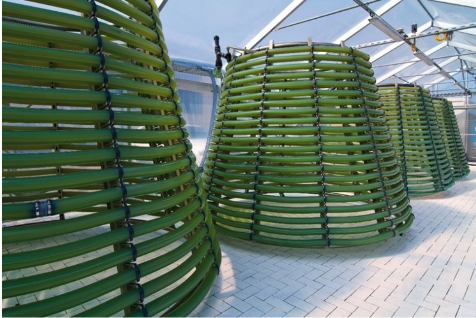
Figure 2.3. Indoor horizontal tubular photobioreactor at GICON® [Public Resource – Image Licence CC BY 4.0]
