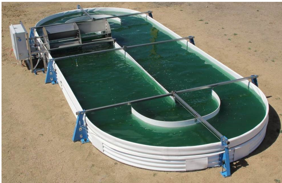
Figure 2.1. Plan view of a raceway pond Adapted from [9] [Public Resource – Image Licence CC BY 4.0]
