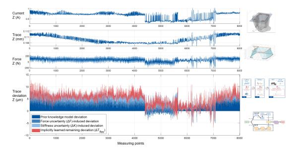
Figure 14: Deviation distribution along the measuring path.
