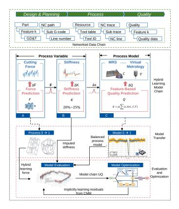
Figure 6: Implementation architecture for the hybrid learning digital twin modeling.
