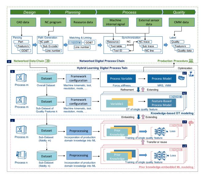
Figure 3: The modeling framework of hybrid learning-based DT for manufacturing process on the basis of the networked digital process chain. a: the data processing procedure for achieving a networked data chain; b: domain knowledge-based DT modeling of the overall part; b2: domain knowledge-based DT modeling of the quality feature on demand; c1: generalized ML modeling for single quality feature; c2: ML modeling for the single quality feature on data with improved quality and fidelity.
