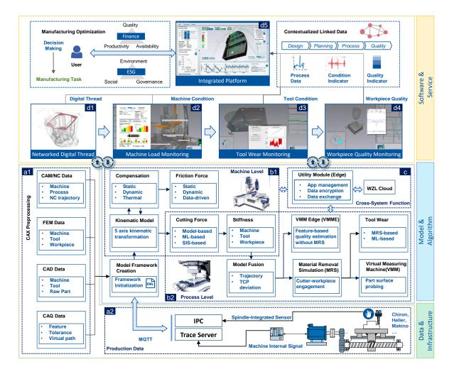
Figure 4: Implementation of digital twin machine tool and machining process at the WZL. ©WZL-RWTH Aachen. Images d2-d4 ©MT Analytics GmbH.
