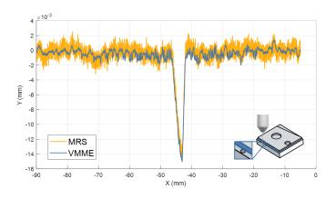
Figure 7: Comparison of estimated workpiece quality using the MRS and VMME.
