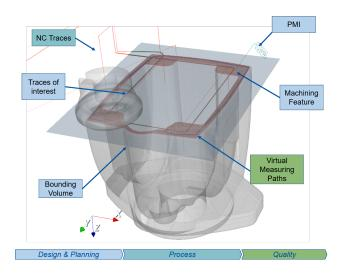
Figure 8: The feature-based digital thread of contextualized metadata sources across the manufacturing procedure: design, planning, NC process, and quality inspection.
