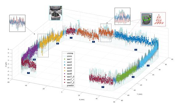
Figure 12: DT results with UQ. Measured and modeled flatness of the selected surface.
