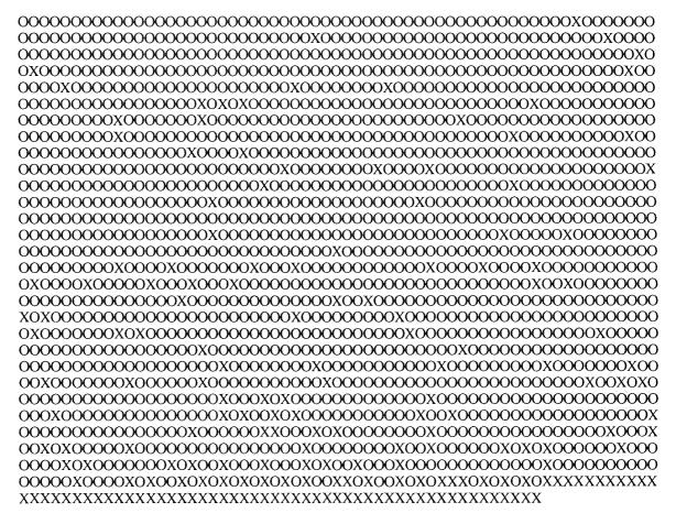
The simulated copolymer contains 1800 HEMA units and 200 EGDMA units
