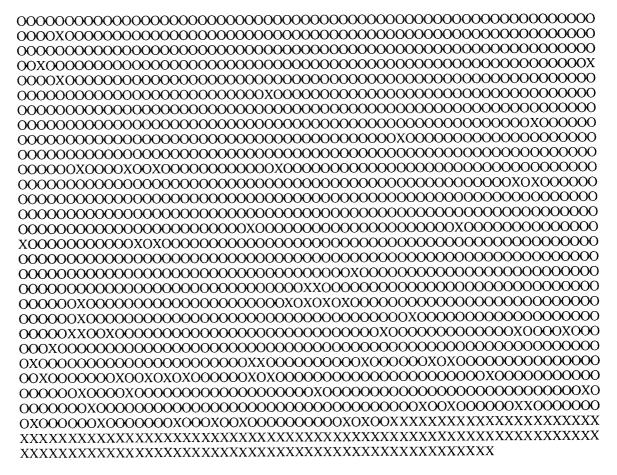
The simulated copolymer contains 1800 HEMA units and 200 TAR units
