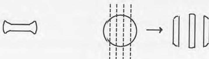
Figure 4.1 Two alternative specimen configurations for samples cut from a contact lens
