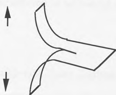
Figure 2.3 Specimen configuration for trouser tear tests
