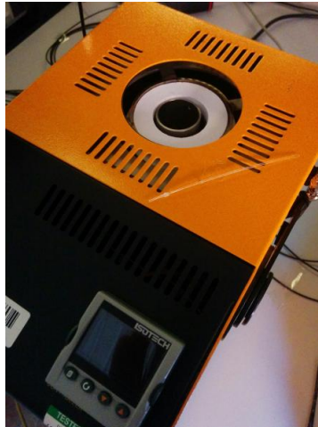
Figure 1. Photograph of the dry block calibrator and the POF sample.
