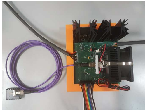
Fig. 2. (a) HPLD optical spectrum; (b) Photograph of the GIPOF based power delivery system.
