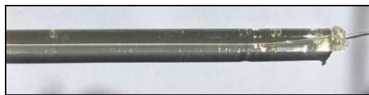
Figure 4. Example of a circular collagen coating around a POF
