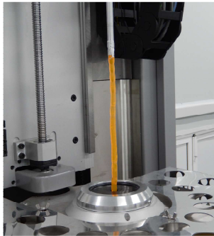
Figure 1. Photograph of the preform settled in the drawing tower.
