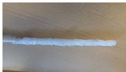
Figure 4. Bubble formation in a TOPAS cane after drying above 70 °C.
